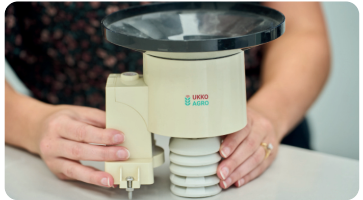
Ukko Agro weather station used for predictive modelling.
